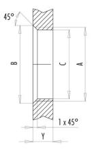
Installation direction: o-ring sits on chamfer.
